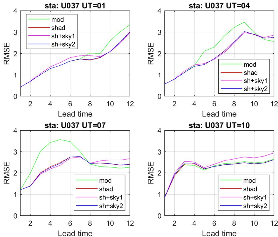
**Fig. 1.** Root mean square errors (RMSE, in degrees) of the road surface temperature forecast for the RWS U037, which is exposed to shading. The RMSE values were calculated for the whole period January-March 2017. They are plotted in dependence on the lead time up to 12 hours for the forecasts started at 01, 04, 07 and 10 UTC. The coloured lines correspond to the results of model version I (green line), II (red line), III (magenta line), and IV (blue line).
