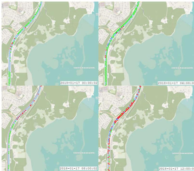
**Fig. 2.** Road surface condition of Ring Road 1 in Helsinki 17.1.2018 ( $T = -5 \text{ degC}$ ). The colours on the map indicates the current road surface condition the same way as in Figure 1.
