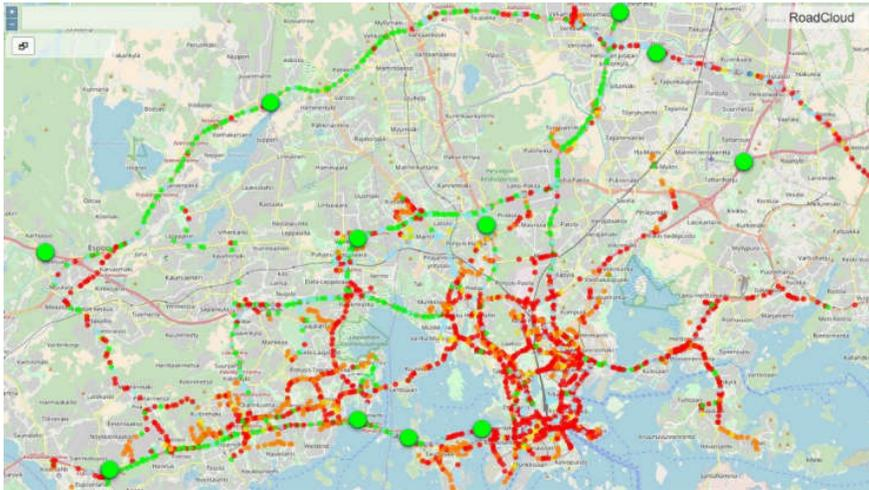
**Fig. 1.** Road network surface condition from mobile measurements (dry - green, light blue - moist, dark blue – wet, red – ice, snow - orange, yellow - slush) and static weather stations (larger circles) indicating dry conditions.
